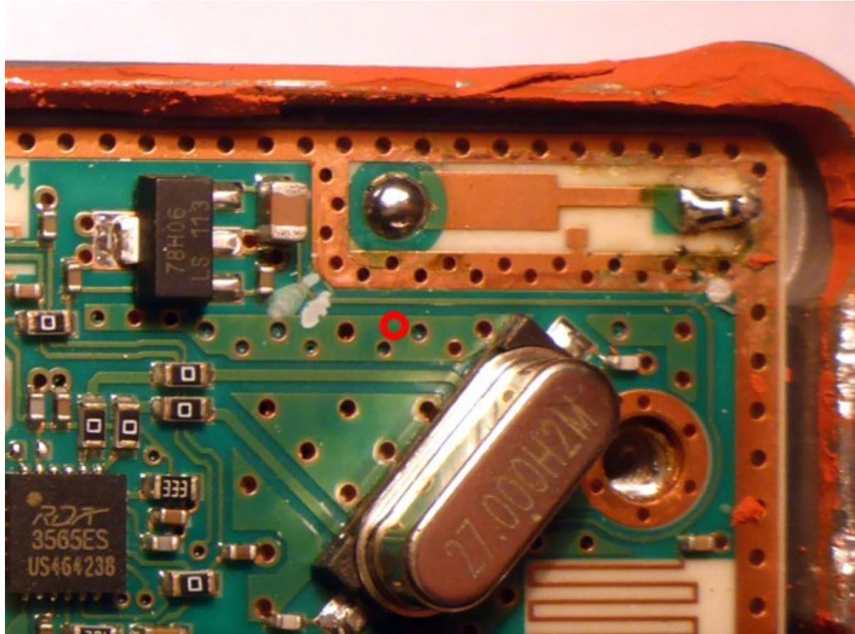
One of the 'vias' that were gained during the disassembly can be reused and guides the 27 MHz signal upwards, where it can be connected to the nearest pad of the crystal. Be sure to check for short circuits after the modification.
