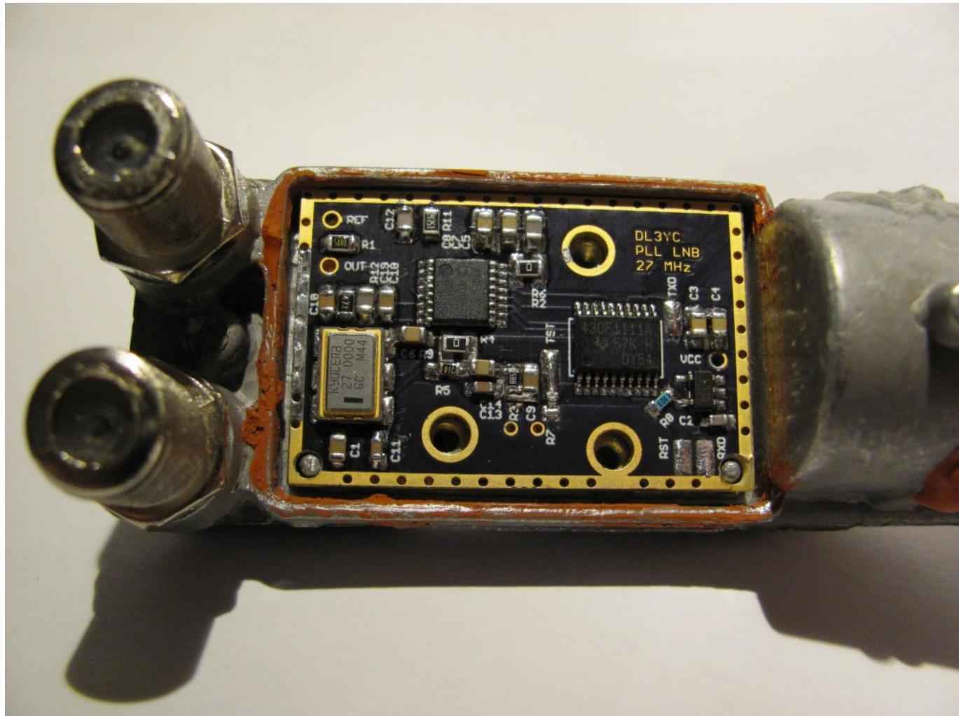
The MSP430F1111 programs the ADF4002 PLL registers and locks the 27 MHz VCXO to the supplied 10 MHz reference input. After successful programming approximately 1.7 V can be measured on the VCXO tuning line.
