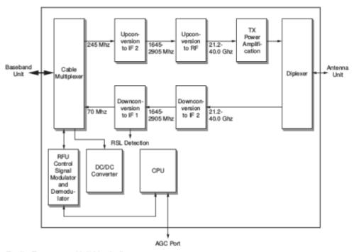
Radio Frequency Unit block diagram
