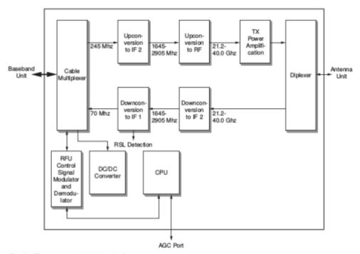
Radio Frequency Unit block diagram
