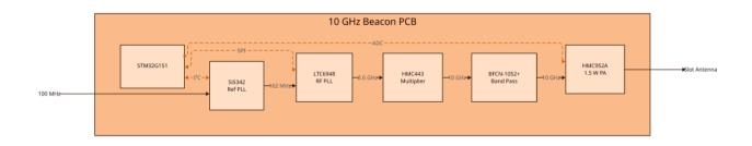
The beacon transmitter accepts an external 100 MHz reference clock provided by a GNSS-disciplined oscillator. GNSS stabilization is the de-facto standard for beacons on 10 GHz and above due to their narrow spacing and small bandwidth. It also enables receiving stations to use the beacon as a frequency reference for aligning their own equipment.
