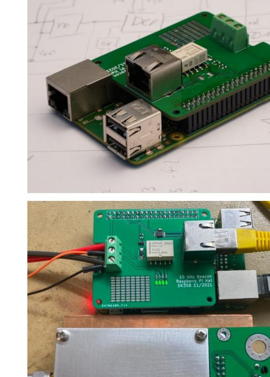
The transmitter and its slot antenna were finally mounted on a large heat sink and placed on a base plate. A 10 GHz circulator was added in-line to avoid damaging the TX in case the return loss of the antenna suddenly degrades due to e.g. temporary water intrusion. An outdoor GNSS antenna was mounted adjacent to the transmitter, to be used for the GNSSDO. The whole assembly is enclosed within a (commercial, surplus) fiberglass radome.
