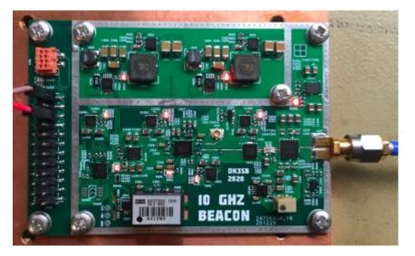
One of the key design features that helps with driving down cost is working with a commercial fourlayer FR4 stackup. These have become ubiquitous and cheap to use, so one supplier (JLCPCB from China) was chosen and their PCB process characterized for RF performance. Two dedicated RF test coupons were designed: Based on the results of long simulations, prototype designs for SMA connector footprints, microstrip, coplanar waveguides etc were designed.
