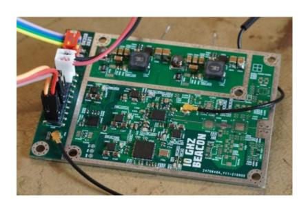
Before going into continuous operation at DB0HDF, the transmitter hard- and software were extensively tested on the lab workbench. The output power, phase noise and spurious performance was first evaluated, with a particular emphasis on varying input voltage conditions. Long supply wires could possibly cause regulator instabilities in final installations, and (resistive) voltage drop could across the cable could cause unexpected input voltage conditions.
