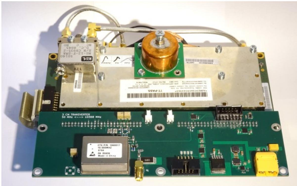
First all the details of the modules were reverse engineered(documented [here](#) in german) and a concept for the usage as a 3cm transverter was worked out. A first prototype was tinkered together and performed very well:
