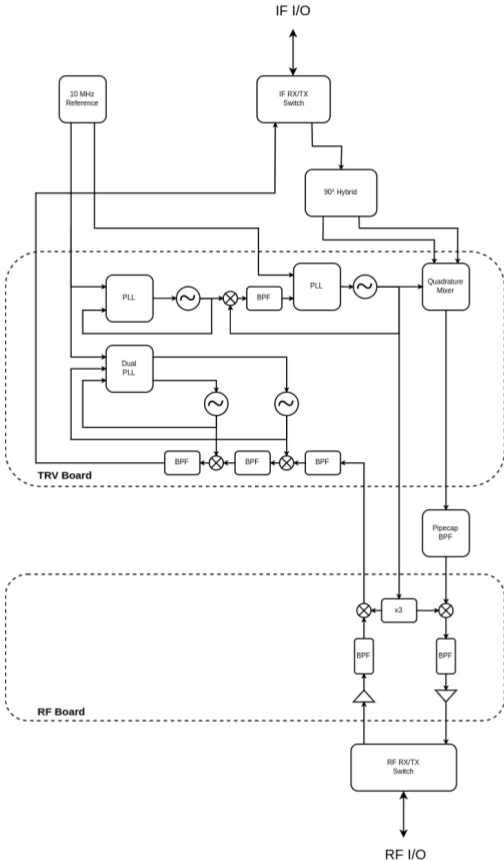
As transceiver IF 50 MHz is used. The transmit path is designed for <1W input power. With a 90° hybrid coupler the quadrature mixer in the transmit section of the transceiver module is used as a image reject mixer to 2.63 GHz. This IF gets filtered externally with a 28mm pipe cap filter to further attenuate the LO and side-band signal (+harmonics). In the first built 0.5 W output power could be reached without additional tuning of the power amplifier. The receiving chain consists of 3
