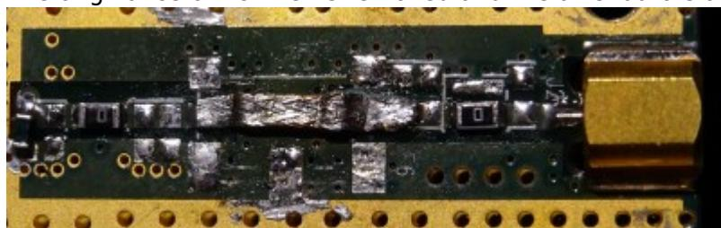
In theory image rejection by the quadrature mixer can be tuned to -60 dBc or better but thermal drift limits the image rejection to about -50 dBc. A pipecap filter with a 28 mm pipecap is added between the transverter board and the rf board.
