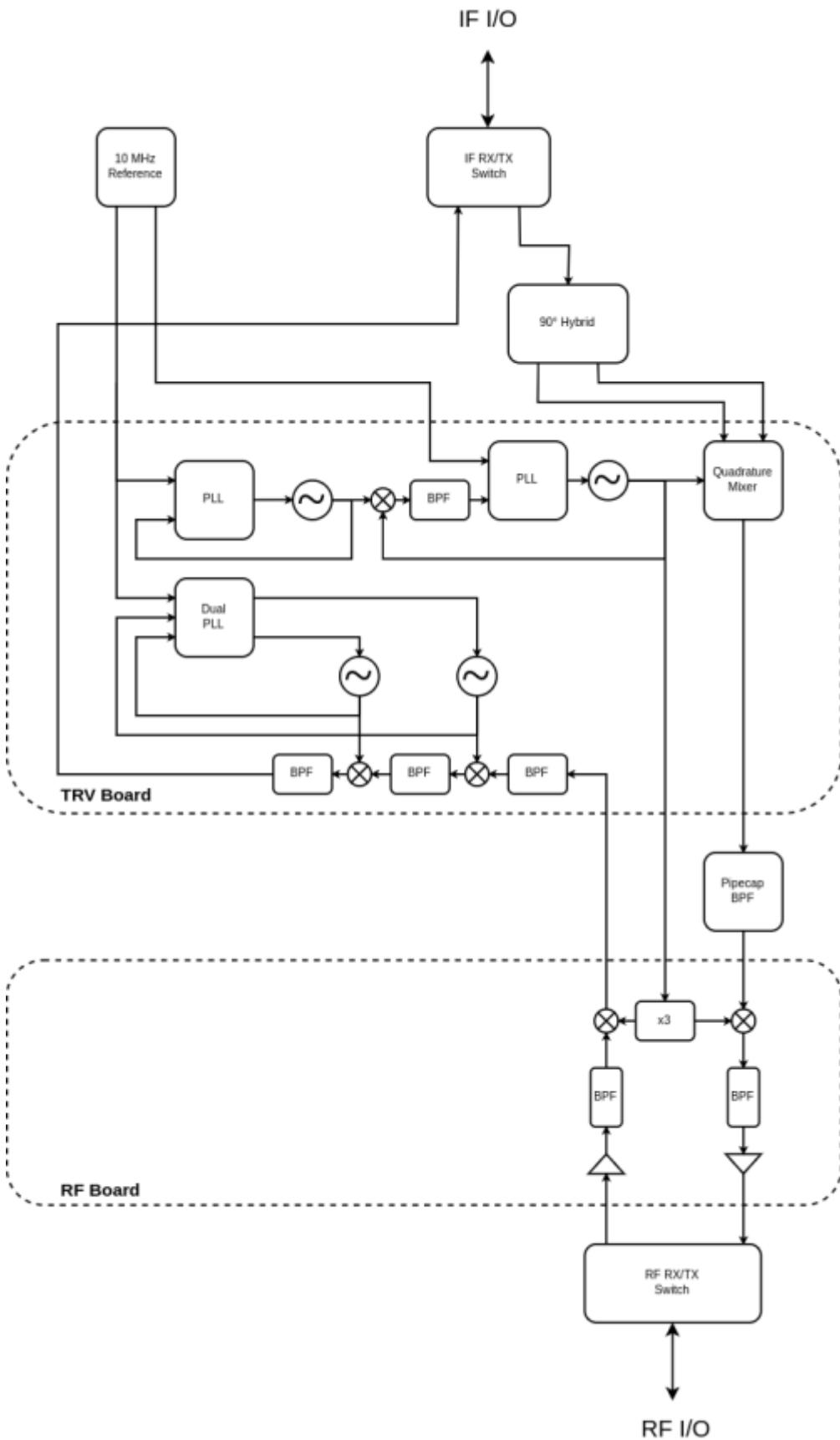
As transceiver IF 50 MHz is used. The transmit path is designed for <1W input power. With a 90° hybrid coupler the quadrature mixer in the transmit section of the transceiver module is used as a image reject mixer to 2.63 GHz. This IF gets filtered externally with a 28mm pipe cap filter to further attenuate the LO and side-band signal (+harmonics). In the first built 0.5 W output power could be
