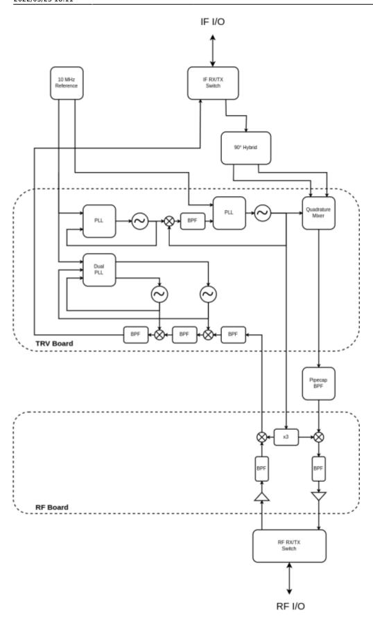
As transceiver IF 50 MHz is used. The transmit path is designed for <1W input power. With a 90° hybrid coupler the quadrature mixer in the transmit section of the transceiver module is used as a image reject mixer to 2.63 GHz. This IF gets filtered externally with a 28mm pipe cap filter to further attenuate the LO and side-band signal (+harmonics). In the first built 0.5 W output power could be
