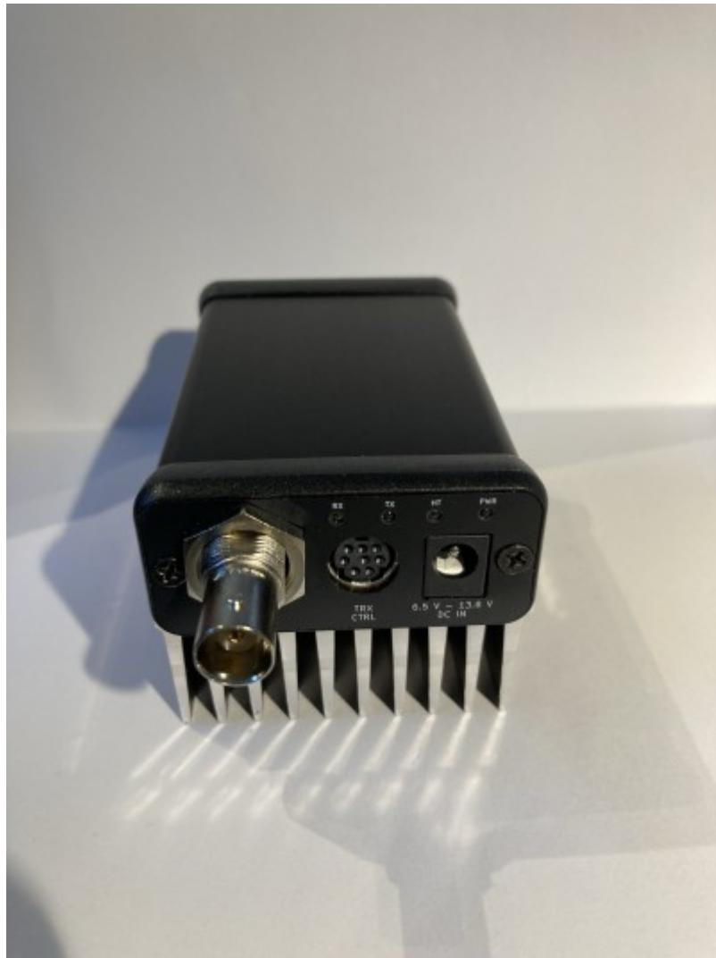
Front and back panels are low-cost PCBs with black solder mask and white silk screen. LEDs are placed on the back panel to show the current state.
