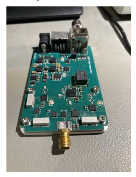
In transmit mode the 7.5 W of heat is dissipated. For proper heat sink the PCB is directly connected to
