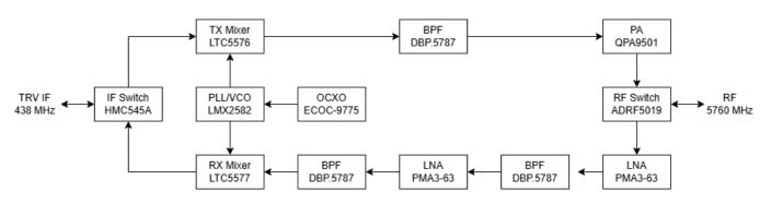
The transverter is designed for an UHF intermediate frequency (IF) and is compatible to the 70 cm all-mode transceiver Yaesu FT817 with 100 mW output power. It handles all the sequencing and transmitter protection through the accessory connector. The local oscillator (LO) uses an ovenized oscillator (OCXO) as stable frequency reference in a small footprint.
