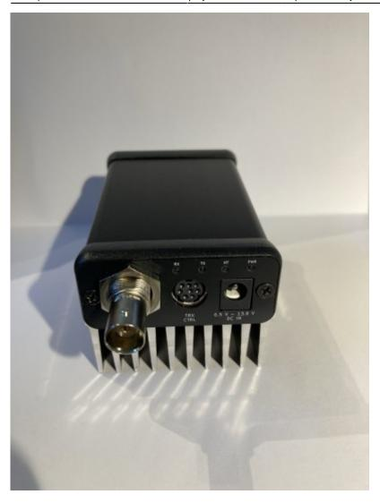
Front and back panels are low-cost PCBs with black solder mask and white silk screen. LEDs are on the back panel to show the current state: heating, receiving, transmitting. The LEDs have different meaning depending on the transceiver's state.
