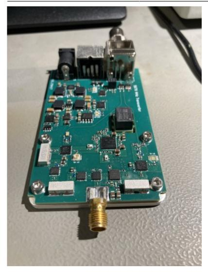
In transmit mode 7.5 watts of heat is dissipated. For proper heat sink the PCB is directly connected to the housing with attached heatsink.
