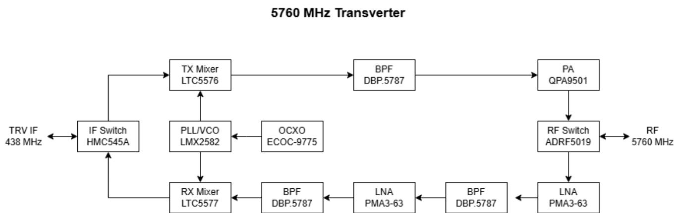
The transverter is designed for an UHF intermediate frequency (IF) and is compatible to the 70 cm all-mode transceiver Yaesu FT817 with 100 mW output power. It handles all the sequencing and transmitter protection through the accessory connector. The local oscillator (LO) uses an ovenized oscillator(OCXO) as stable frequency reference in a small footprint.
