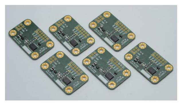
The PCB can be wired as shown below: A front panel toggle switch is used to enable/disable the CW generation, and two audio jacks can be wired to the front panel and the transceiver. This allows using a manual/paddle keyer in addition to this circuit. The PCB simply pulls the "tip" contact to ground to key the TRX.
