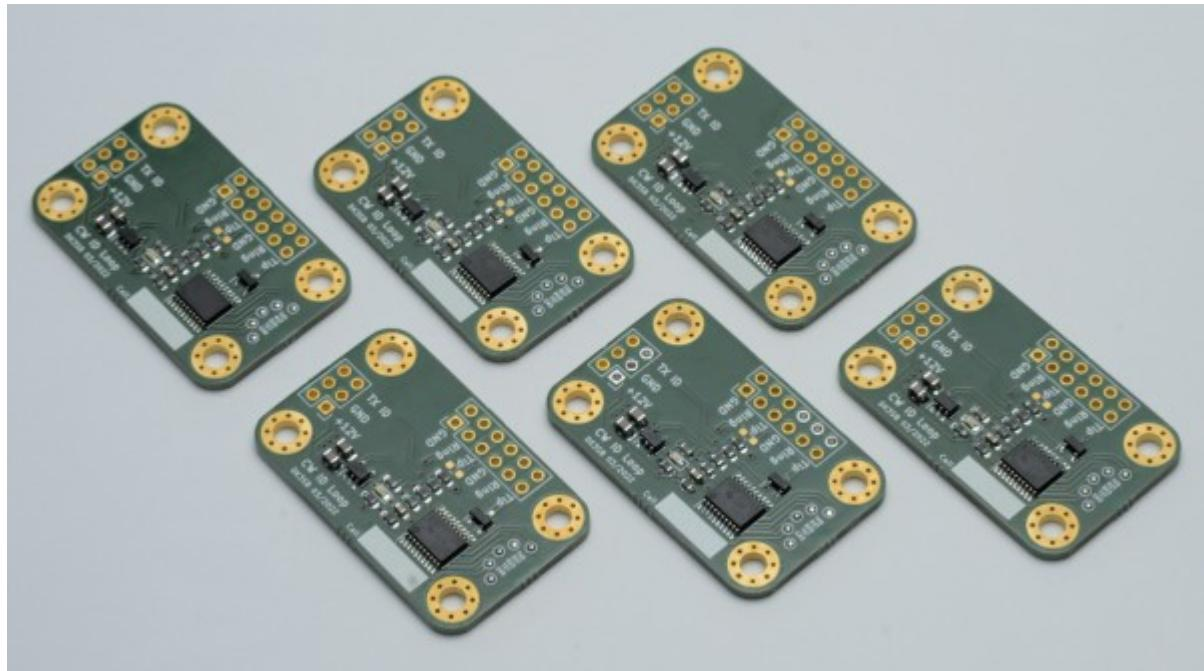
The PCB can be wired as shown below: A front panel toggle switch is used to enable/disable the CW generation, and two audio jacks can be wired to the front panel and the transceiver. This allows using a manual/paddle keyer in addition to this circuit. The PCB simply pulls the „tip“ contact to ground to key the TRX.
