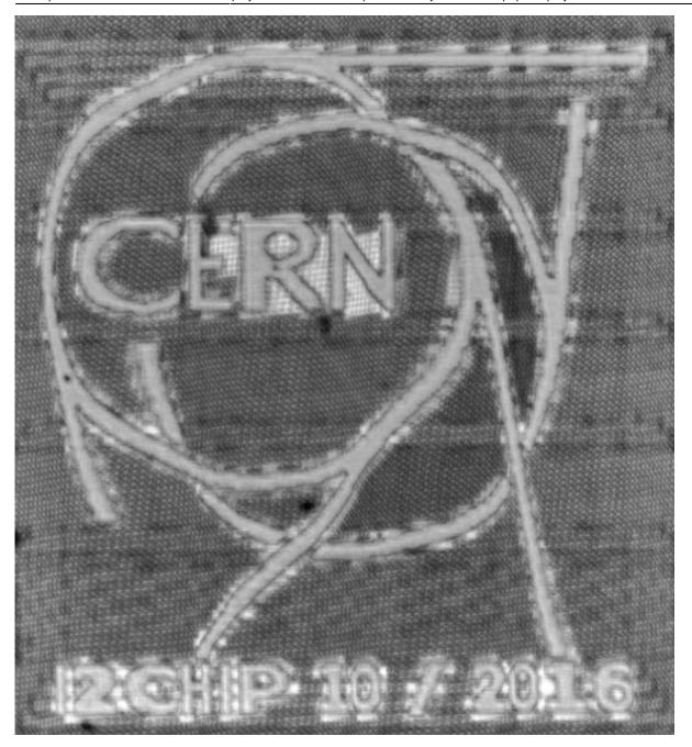
This picture shows some of the aforementioned nonlinearity in one axis, which introduces periodical distortions in the image. These could be corrected in principle, but I didn't bother. The nice CERN logo was placed on the top metal layer, and is composed of many small pixels that are on the order of a few micrometers large.
