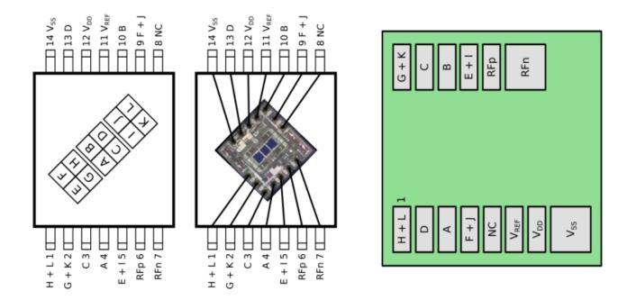
The output producing negative voltages is not considered to be useful in the final application, while the differential output pair is likely a summed output of the four inner quadrants (the RF output). With the assignment of pins to diode quadrants done, the OPU could be modified to fan-out the required connections to custom electronics
