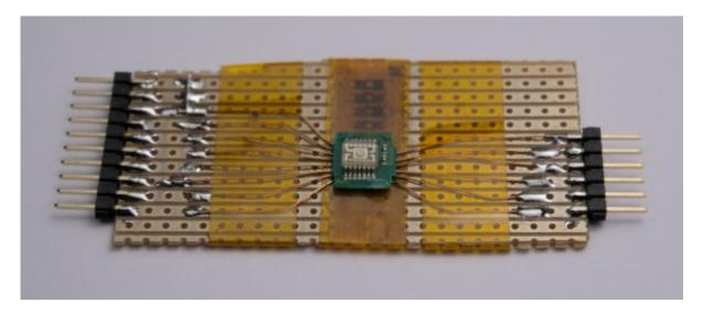
Initial pinout probing revealed only the power supply pins and a number of analog output voltages, however no datasheet for a PDIC with matching pinout could be found online. To be able to re-use this component, a little reverse-engineering effort was started.
