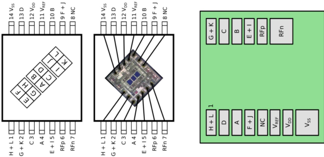
The output producing negative voltages is not considered to be useful in the final application, while the differential output pair is likely a summed output of the four inner quadrants (the RF output). With the assignment of pins to diode quadrants done, the OPU could be modified to fan-out the required connections to custom electronics
