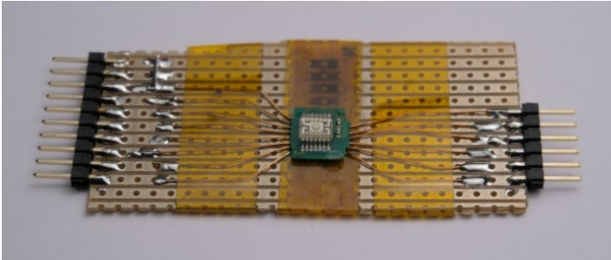
Initial pinout probing revealed only the power supply pins and a number of analog output voltages, however no datasheet for a PDIC with matching pinout could be found online. To be able to re-use this component, a little reverse-engineering effort was started.
