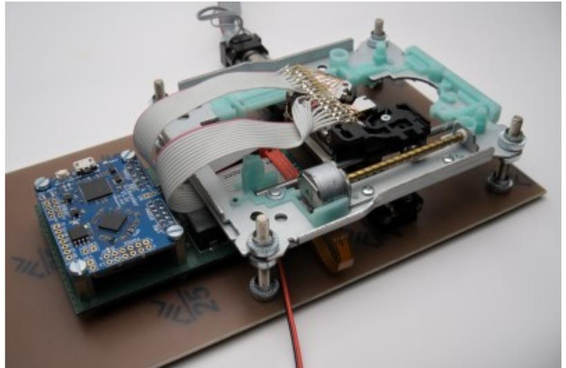
Due to an abundance of one specific type of DVD drives, plans were made to give a useful afterlife to these devices. A laser scanning microscope seemed to be the most useful project.
