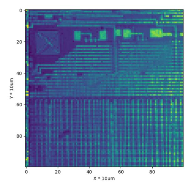
Higher resoultion scan of the same device EPROM, scan area  $500 \times 500$  um. The two routing layers can be seen above one another. (Picture Below)
