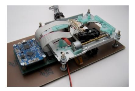
Due to an abundance of one specific type of DVD drives, plans were made to give a useful afterlife to these devices. A laser scanning microscope seemed to be the most useful project.
