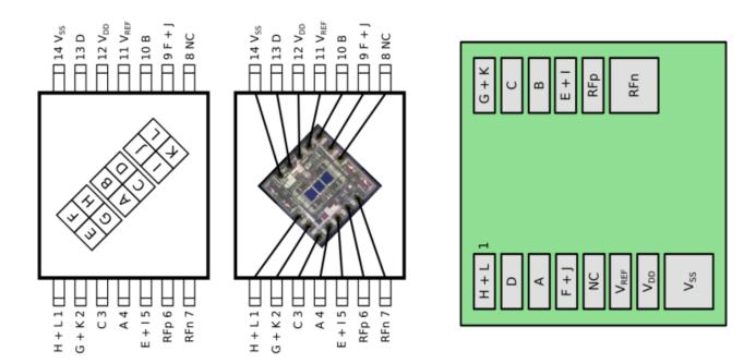
The output producing negative voltages is not considered to be useful in the final application, while the differential output pair is likely a summed output of the four inner quadrants (the high bandwidth RF output). With the assignment of pins to diode quadrants done, the OPU could be modified to fanout the required connections to custom electronics
