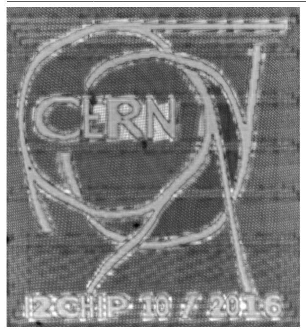
This picture shows some of the aforementioned nonlinearity in one axis, which introduces periodical distortions in the image. These could be corrected in principle, but I didn't bother. The nice CERN logo was placed on the top metal layer, and some of the lower level metals are actually already visible from the top (the vertical and horizontal power distribution stripes are placed on the two metal layers below).
