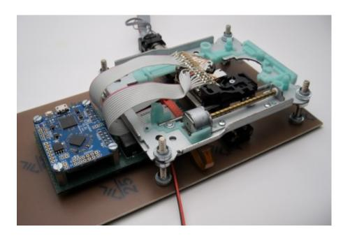
Due to an abundance of one specific type of DVD drives, plans were made to give a useful afterlife to these devices. A laser scanning microscope seemed to be the most useful project.
