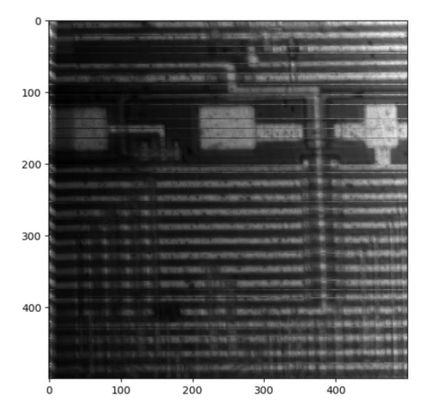
Scan of an I2C test chip from my colleague Szymon (fabricated in 65nm CMOS, picture below). Scan area 1x1mm.
