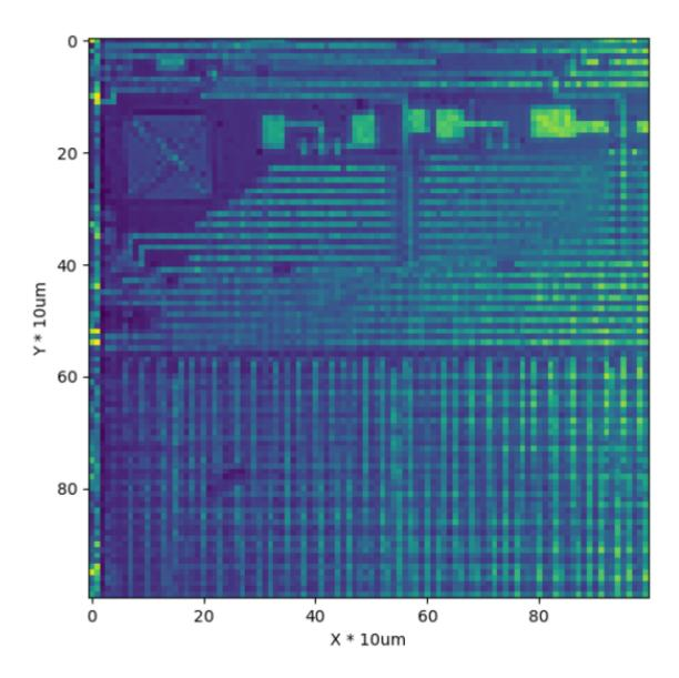
Higher resolution scan of the same device EPROM, scan area  $500 \times 500$  um (top right of previous image). The two routing layers can be seen above one another. (Picture Below)
