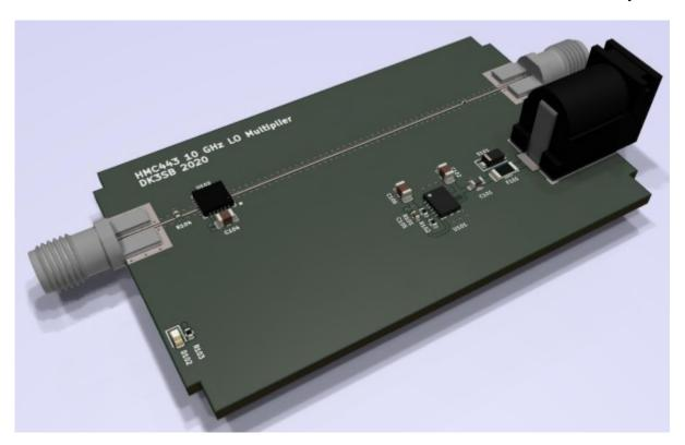
The complete device can be built for below 100 € including the PCBs, which can be considered a nice low-cost alternative to a standalone generator for the 10 GHz range, especially when a 2.5 GHz generator is already available.
