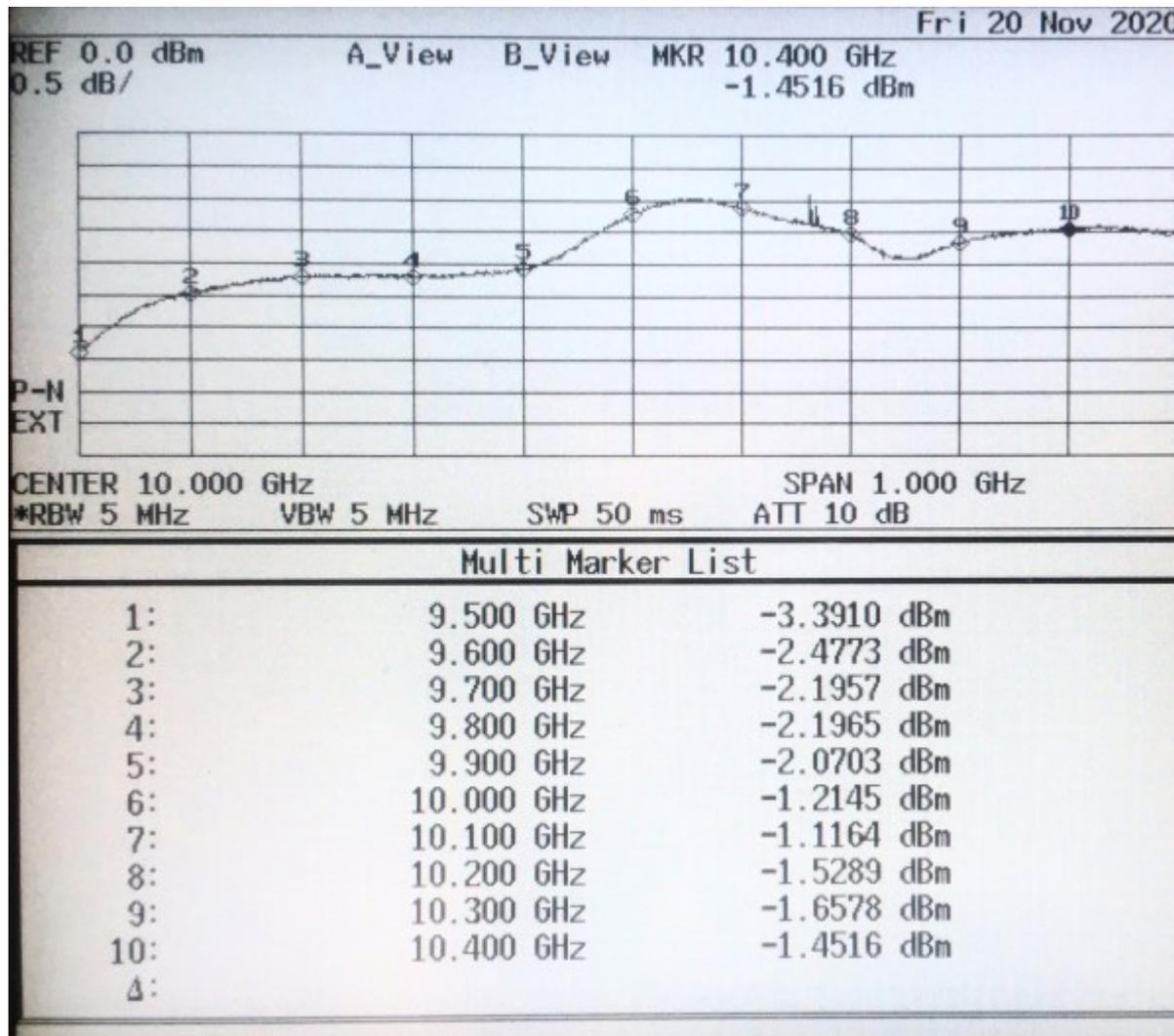
Spectral content was verified at 10.368 GHz to be in line with the datasheet typical values:
