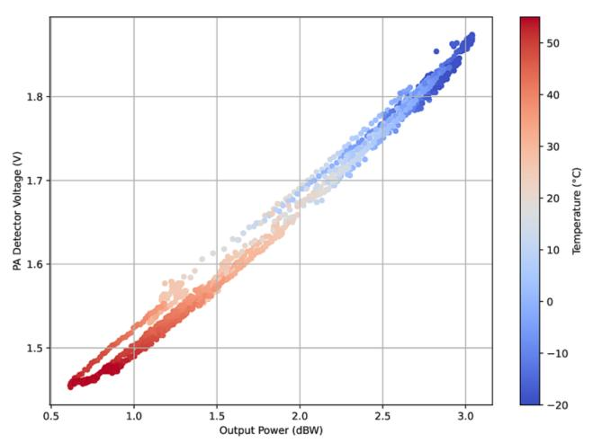
Across the full temperature range, the output power was found to vary by about 2.5 dB. This is not untypical for a fixed gate voltage design without temperature compensation. The negative temperature coefficient ensures there is no thermal runaway at high temperatures, and with a peak RF output power of 2 W at -20°C, there is enough operational margin for some reduction at higher temperatures, aging, etc.
