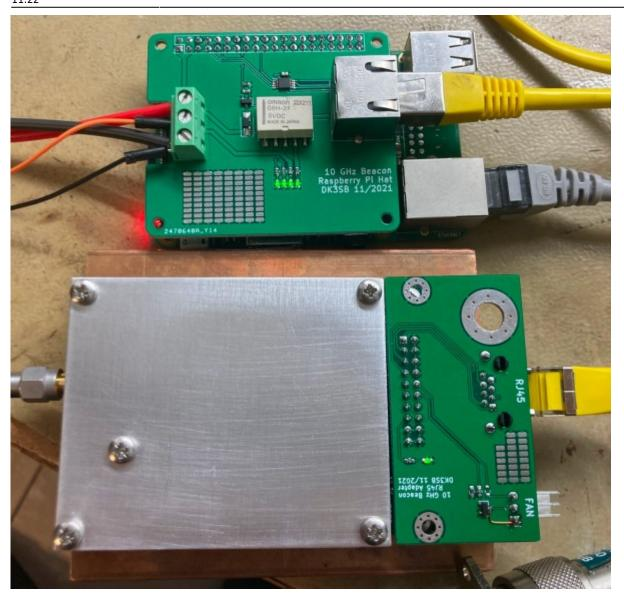
The transmitter and its slot antenna were finally mounted on a large heat sink and placed on a base plate. A 10 GHz circulator was added in-line to avoid damaging the TX in case the return loss of the antenna suddenly degrades due to e.g. temporary water intrusion. An outdoor GNSS antenna was mounted adjacent to the transmitter, to be used for the GNSSDO. The whole assembly is enclosed within a (commercial, surplus) fiberglass radome.
