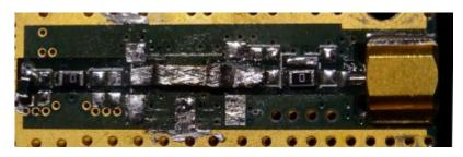
In theory image rejection by the quadrature mixer can be tuned to -60 dBc or better, however thermal drift limits the image rejection to about -50 dBc. A pipecap filter (constructed from a 28 mm pipecap) is therefore inserted between the transverter board and the RF board. It connects in-line using the external MCX connectors.
