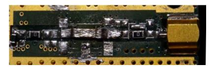
In theory image rejection by the quadrature mixer can be tuned to -60 dBc or better, however thermal drift limits the image rejection to about -50 dBc. A pipecap filter (constructed from a 28 mm pipecap) is therefore inserted between the transverter board and the RF board. It connects in-line using the external MCX connectors.
