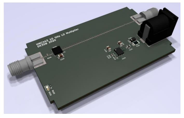
The complete device can be built for below  $100 \in$  including the PCBs, which can be considered a nice low-cost alternative to a standalone generator for the 10 GHz range, especially when a 2.5 GHz generator is already available.
